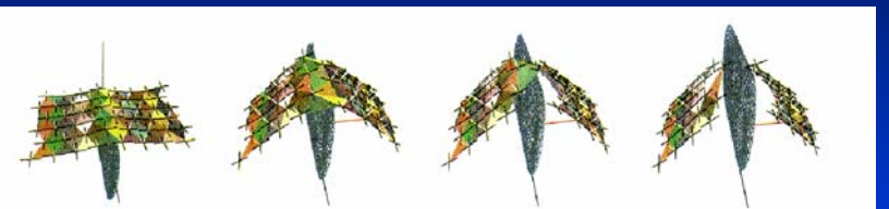
Figure 6: Cutting a surface into two. The movement of the knife edge pushes the particles in the two surfaces apart.
