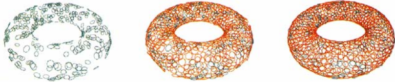
Figure 9: Surface interpolation through a collection of 3-D points. The surface extends outward from the seed points until it fills in the gaps and forms a complete surface.
