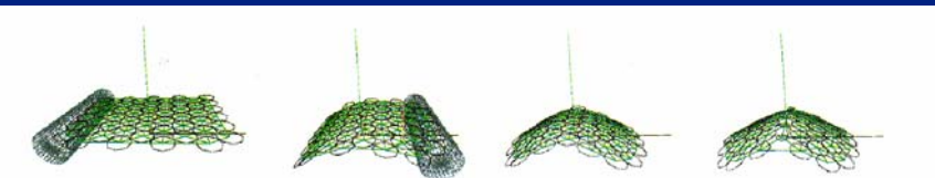
Figure 7: Putting a crease into a surface. The center row of particles is turned into unoriented particles which ignore smoothness forces.
